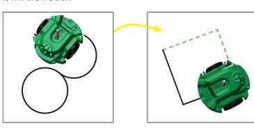
**NOTE:** Just like handwriting, each S3 drawing will be recognizable but unique every time you run a program. Variations occur as battery charge changes, motors warm up, and wheel joints relax with use over time.
